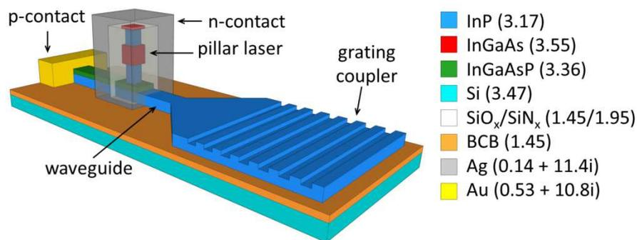
Figure 1. Schematic of a metal-cavity nanolaser coupled to an InP-membrane waveguide connected to a grating coupler. The refractive index of each material at 1.55  $\mu\text{m}$  is shown in parenthesis.
