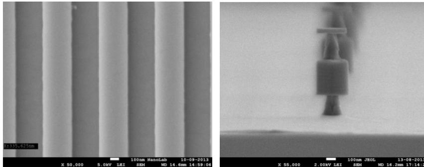
Figure 3. Left: Top view of a typical grating coupler. Right: Pillar with undercut fabricated using the solution H<sub>2</sub>O:H<sub>3</sub>PO<sub>4</sub>:HCl.
