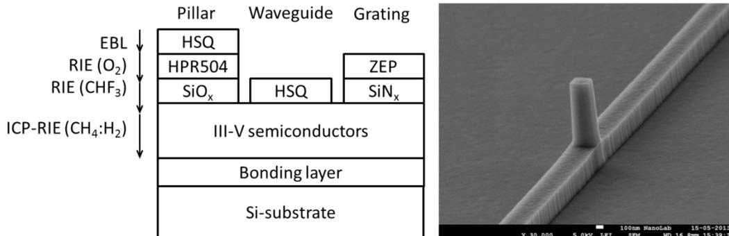
Figure 2. Left: Processing schemes to fabricate the nanostructures. The top layer of each lithographic scheme is always defined by EBL and development. Right: Pillar after waveguide etching and removal of hardmasks.
