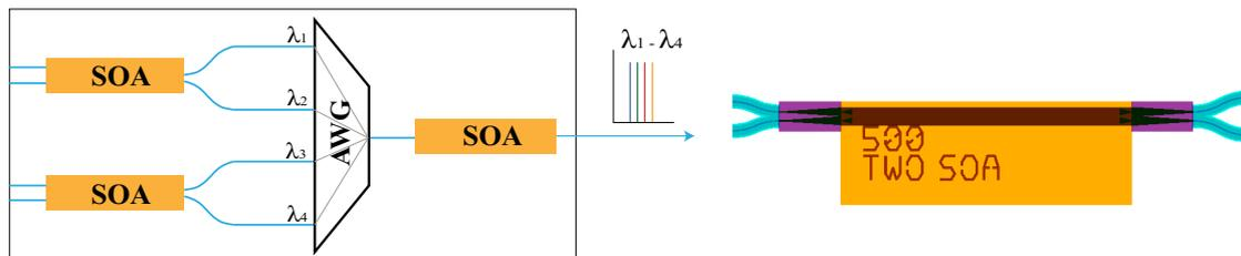
Fig. 1. Schematic of an AWG-based laser (*left*) and mask layout of the double-waveguide SOA (*right*).
