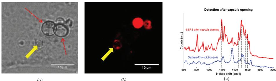
Fig. 3: Illustration of the label-free detection of dextran-rhodamin.  $\text{Si}_3\text{N}_4$  chips and (a) Human fibroblast cell containing three dextran-rhodamin loaded capsules and two gold coated SiN chips (red dashed arrows).(b) Fluorescence signal after opening one capsule (yellow arrow) (c) SERS spectra measured on top of the SiN chips after capsule release (red) and reference spectrum of dextran-rhodamin (blue).
