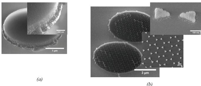
Fig. 1: SEM images of  $\text{Si}_3\text{N}_4$  chips coated with colloidal gold nanoparticles adsorbed to the  $\text{Si}_3\text{N}_4$  surface (a) and nanotriangles fabricated through nanosphere lithography.
