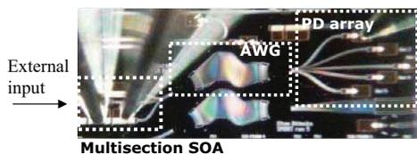
Figure 4 Microscope photo of the realized test structure for on-wafer modal gain characterization. Needles provide the electrical signals needed for the on-wafer characterization.
