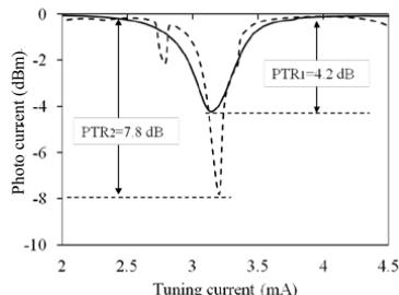
Figure 2 Electrically measured transmission for ring 1 (solid black) and for ring 2 (dashed black).
