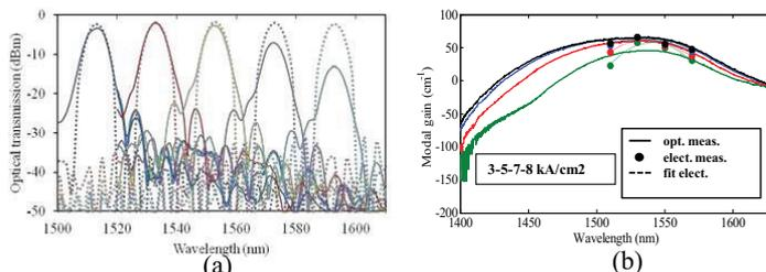
Figure 5 Simulated (dotted) vs. measured (solid) TE transmission spectra of the AWG in (a). Optically vs. electrically measured modal gain for different current densities in (b).
