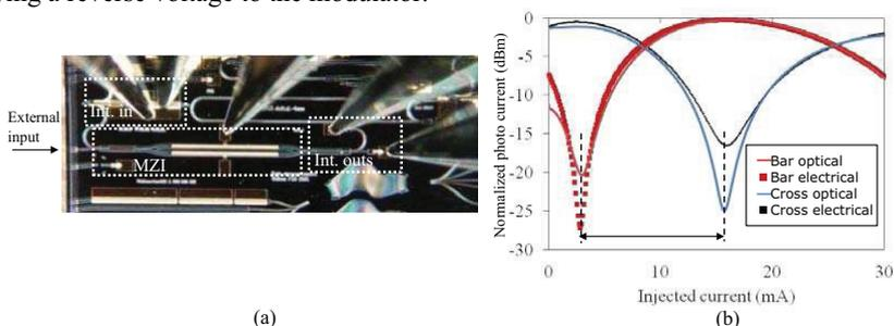
Figure 3 Microscope photo of the realized test structure during on-wafer phase efficiency characterization (a), and electrically measured (dotted) vs. optically measured (solid) phase efficiency (b).
