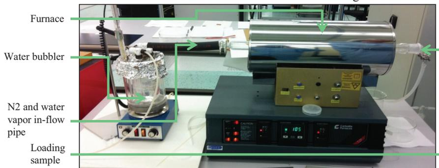
Fig.2: Experimental setup for oxidation process.
