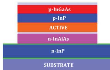
Fig.1: Mesa structure for active component fabrication.
