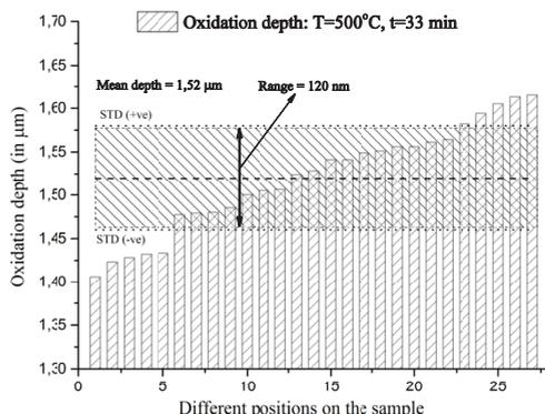
Fig.5: Plot of oxidation depth at various positions on the sample.
