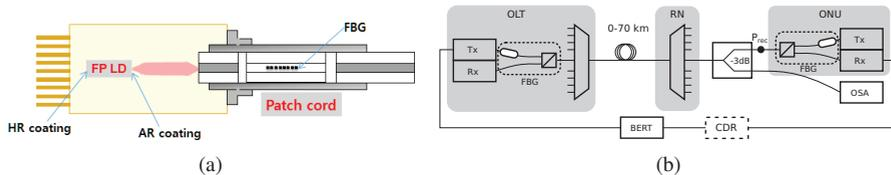
Fig. 1. (a) Schematic representation of the transmitter. Picture courtesy of MEL Telecom. (b) Schematic representation of the experimental setup. BERT denotes the bit error rate tester, CDR the clock-data recovery if present, FBG the pluggable patch cord including a fiber Bragg grating and C/L band splitter.
