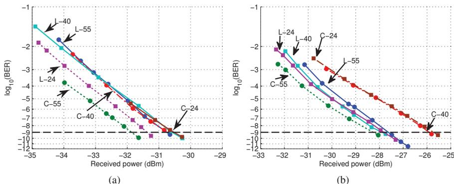
Fig. 3. BER curve of: (a) 1.25 Gbps data transfer back-to-back for six wavelength channels (b) 2.5 Gbps data transfer over 40 km of fiber for six wavelength channels
