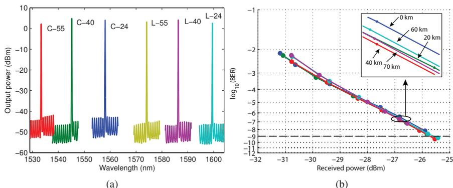
Fig. 2. (a) Spectrum of the six characterized transmitter combinations in ITU-T bands 24, 40 and 55 in the C and L bands, (b) BER curve of 2.5 Gbps data transfer over distances ranging from 0 to 70 km for channel C-24.
