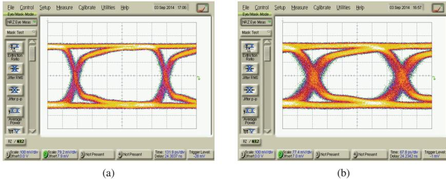
Fig. 4. Eye diagrams of: (a) 1.25 Gbps transfer over 20 km of fiber (b) 2.5 Gbps transfer over 40 km of fiber
