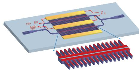
Figure 1: Segmented slot waveguide in a Mach Zehnder configuration.
