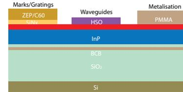
Figure 3: Lithography mask schemes used in the fabrication.
