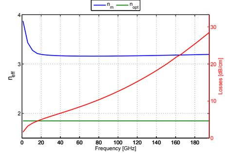
Figure 2: Left axis: RF index and optical index. Right axis: RF losses
