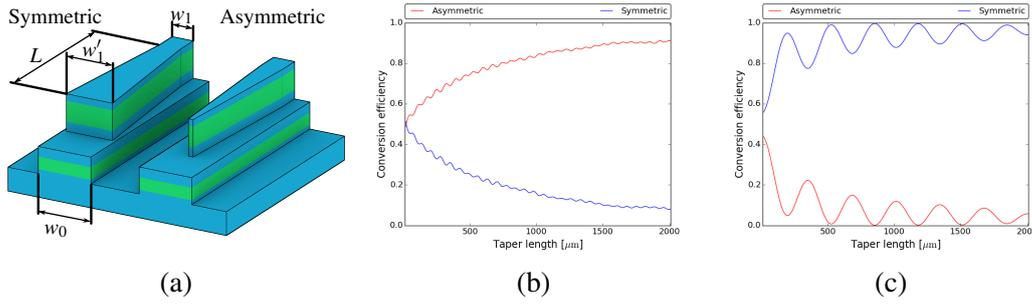
Figure 3: (a) Tapered mode converter for exciting the symmetric and asymmetric super modes. Conversion efficiency as a function of taper length for converters with taper start width of (b)  $w'_1 = 1.0 \mu\text{m}$  and (c)  $w'_1 = 2.2 \mu\text{m}$ .
