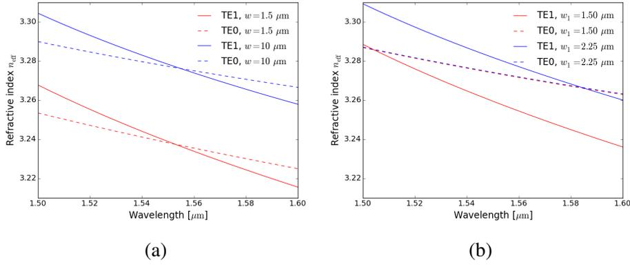
Figure 2: Dispersion relation of TE0 and TE1 modes for (a) single width waveguide ( $w = w_0 = w_1$ ,  $1.01 \mu\text{m}$  upper core thickness) and (b) dual width waveguide.
