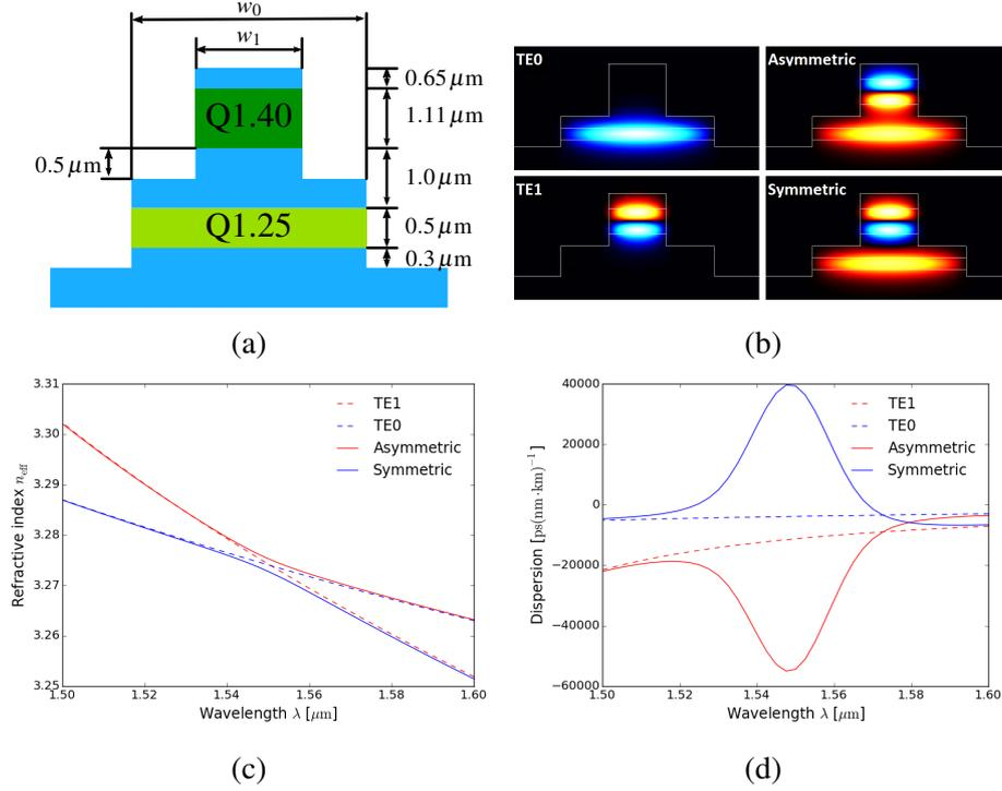
Figure 1: (a) Crosssections of dual layer, dual width InP/InGaAsP based waveguide and (b) corresponding horizontal electric field distribution for the uncoupled modes (TE0 and TE1) and the super modes (asymmetric and symmetric.) (c) Dispersion relation and (d) calculated dispersion for the same modes.
