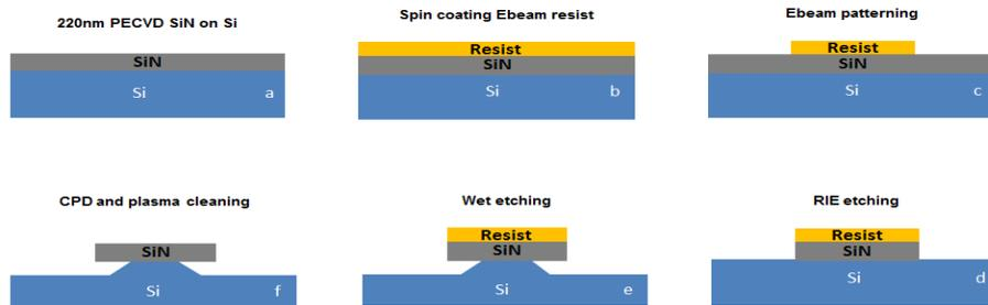
Fig. 5. Schematics of the fabrication flow of ultra-compact grating coupler
