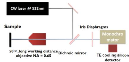
Fig. 7. Schematics of the measurement setup
