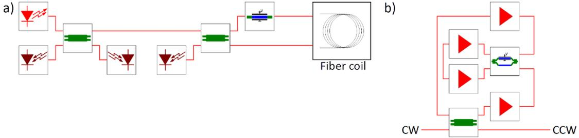
**Fig. 1. Circuit scheme of an integrated interrogator for an interferometric fiber-optic gyroscope (a) and an integrated ring laser gyroscope (b).**
