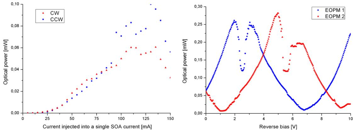
**Fig. 4. Measured laser power characteristics versus current injected into a single SOA section (left) and versus reverse bias applied to the EOPM sections (right).**
