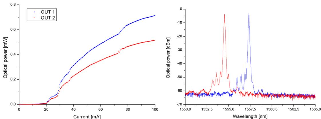
**Fig. 3. Measured laser power characteristic (left) and output spectra (right) of the DBR laser of the IFOG integrated interrogator.**
