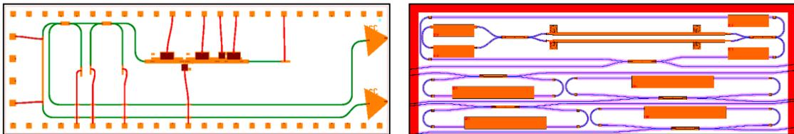
**Fig. 2. Mask layout of the integrated interrogator for an interferometric fiber optic gyroscope (left) and the integrated ring laser gyroscope (right).**
