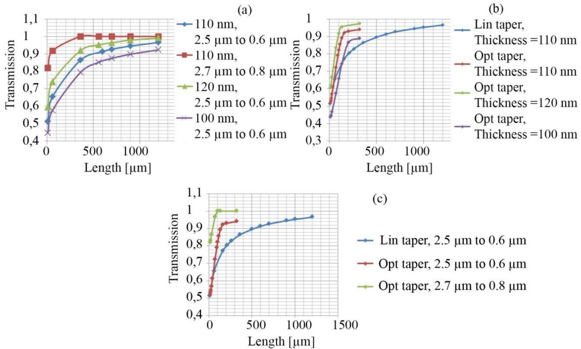
Fig 3: (a) Linear taper, tolerance tests; (b) Optimized Taper with proposed length= 900 μm: tolerance tests for thickness ( $\pm 10$  nm); (c) Optimized taper with proposed length= 900 μm: tolerance tests for widths;
