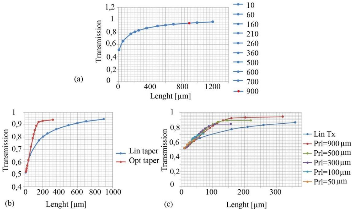
Fig 2: (a) Convergence test for linear taper in case of 2.5  $\mu\text{m}$  to 0.6  $\mu\text{m}$  widths; (b) Comparison of transmission values between optimized and linear structure; (c) Comparison of transmission values between several proposed lengths.
