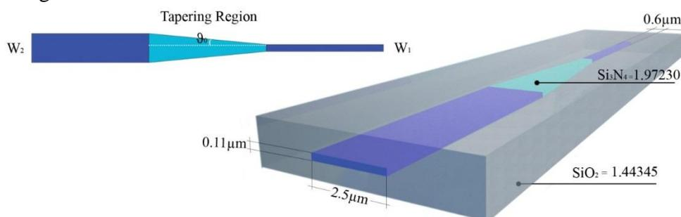
Fig. 1: Top view and 3D representation of the linear structure.
