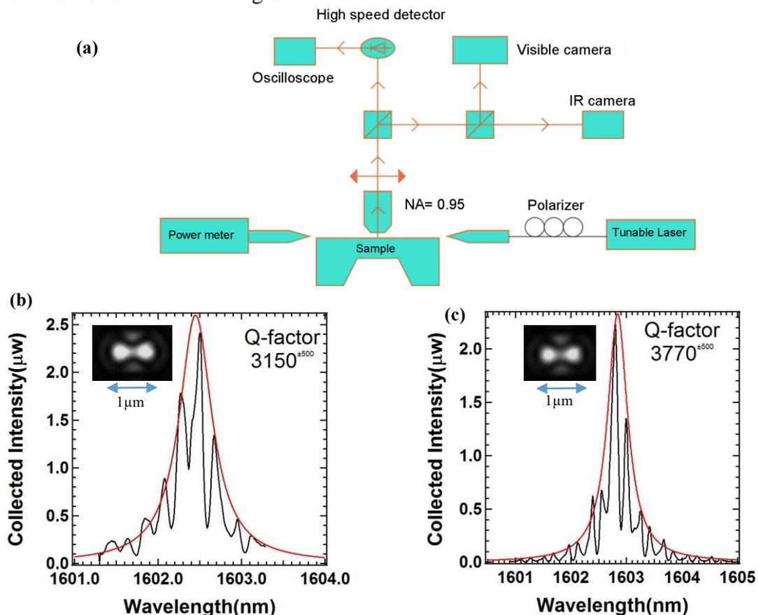
Figure 2. (a) Schematic of the experimental apparatus used for PhC characterization. (b), (c) transmission spectra of substrate-less PhC cavity and cavity without substrate removal respectively. (Inset- intensity pattern of the cavity field at resonance)
