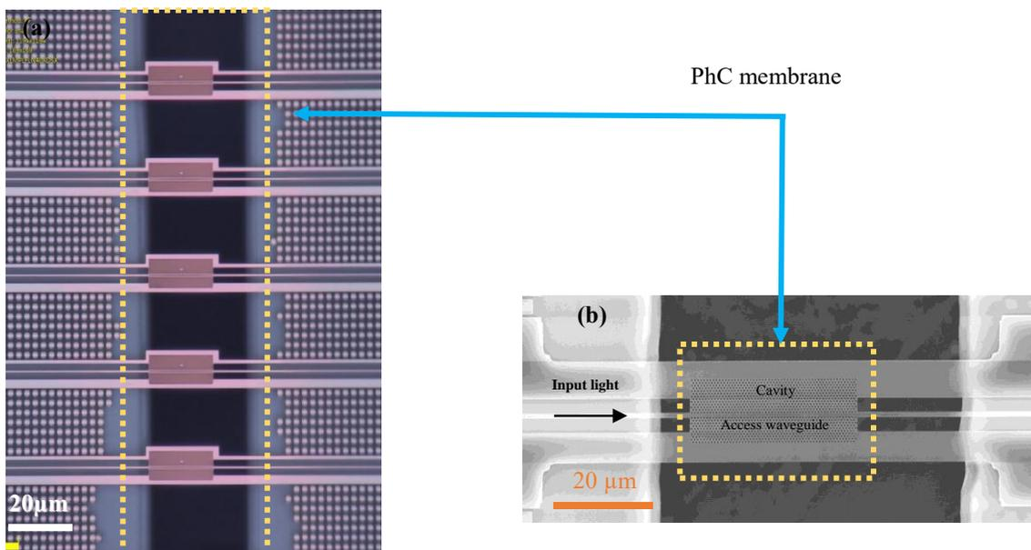
Figure 1: (a) Optical microscope image of substrate-less PhC membrane. (b) scanning electron microscope (SEM) image of PhC membrane (cavity is excited by input light coupled into access waveguide).
