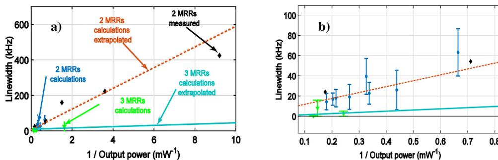
Fig.3 a) Measured linewidth of the laser with 2 MRRs and calculated linewidth for both lasers with 2 MRRs and 3 MRRs; b) zoom in of a)
