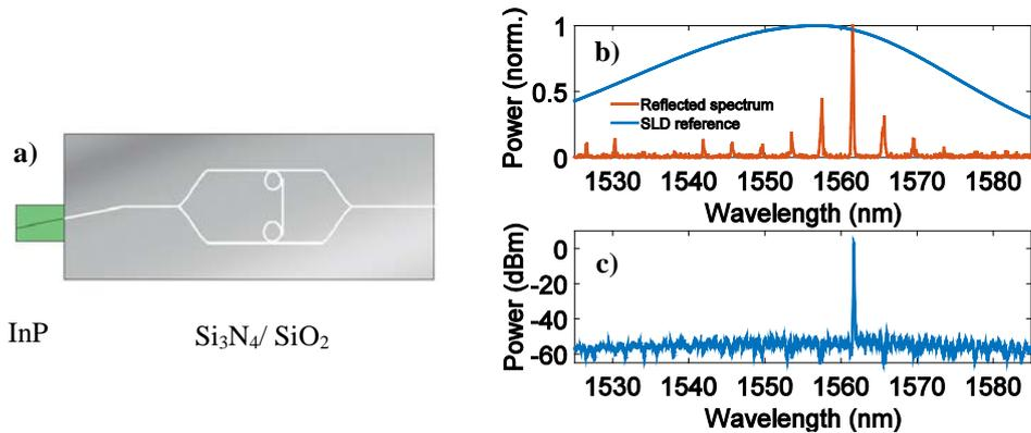
Fig.1 a) Schematic of the hybrid laser with two MRRs; b) the superimposed spectra of the measured reflected power of the double MRR mirror (red) as a function of wavelength and the spectrum of the used superluminescent (SLD) diode (blue), both normalized to their maxima; c) laser spectrum with 50 dB SMSR. The measured spectral bandwidth of the oscillating laser mode is 24 kHz (FWHM).
