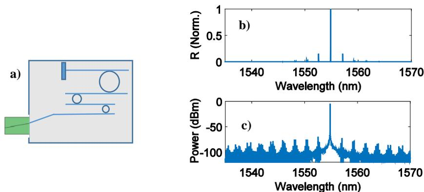
Fig.2 a) Schematic of the hybrid laser with three MRRs; b) the calculated reflectivity as a function of wavelength of the three MRR mirror c) calculated output spectrum shows a SMSR about 50 dB
