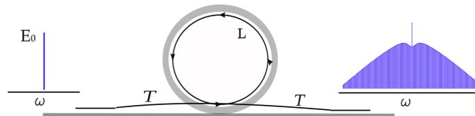
Figure 1: A synchronously pumped fiber cavity.  $T$  is the transmission coefficient of the beam splitter.  $L$  is the length of the fiber.
