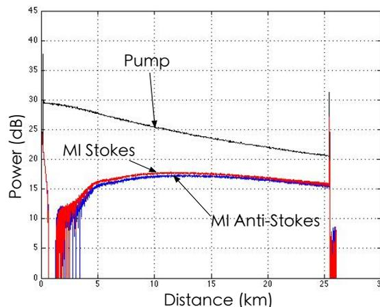
Figure 4: Distributed measurement at the pump, stokes and anti-stoked wavelengths.
