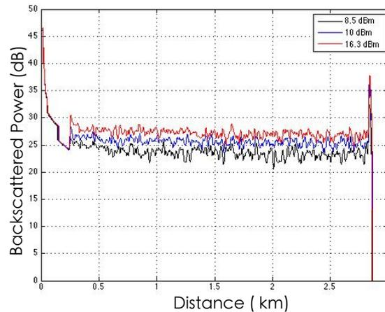
Figure 2: Evolution of the backscattered signal for different average power,
