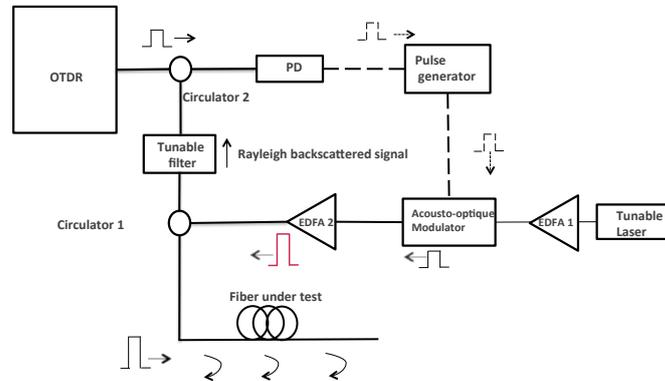
Figure 3: Experimental set up for the distributed measurement of MI
