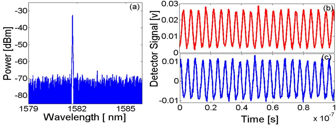
**Figure 2:** While pumping the SRL at 85 mA, gate 3 at 46.7 mA. (a). Optical spectrum in the CW direction. (b). Time trace of the device output in the CW. (c). Time trace of the device output in the CCW.
