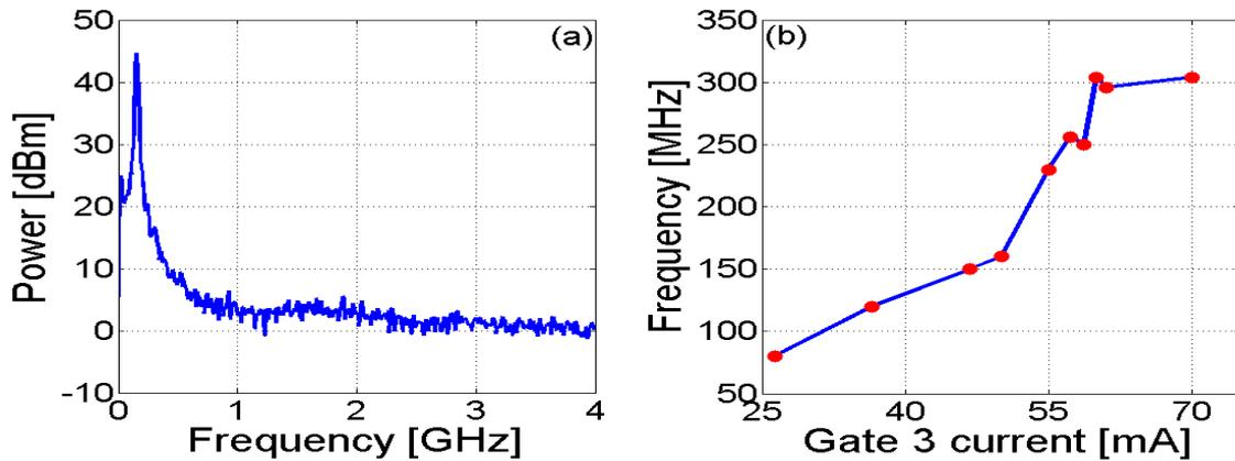
**Figure 3:** (a). Electrical spectrum in the CW direction. (b). Frequency of the oscillations as function of gate 3's current while SRL current is fixed at 85 mA.
