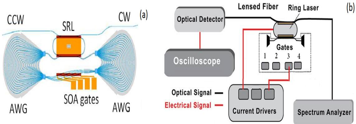
**Figure 1:** (a). Mask layout of the integrated ring laser with filtered optical feedback. (b). Lab setup.
