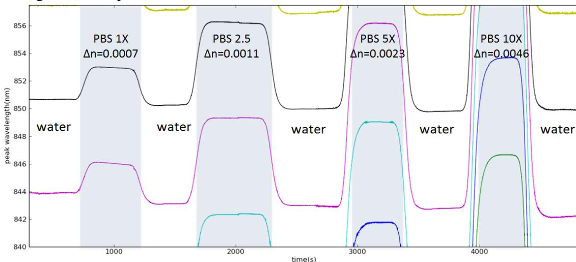
Figure 3: Time evolution of fitted peak wavelengths of Mach-Zehnder interferometer upon exposure of different PBS mixtures alternated with water. Different colored curves correspond to different peaks of the same sensor. The refractive index difference with water of the mixtures is indicated on the figure.
