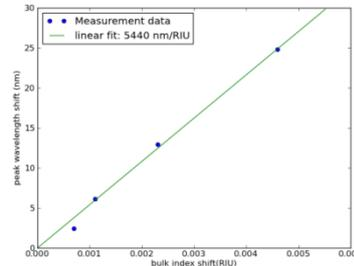
Figure 4: Linear fit of the peak wavelength shift to the bulk index shift
