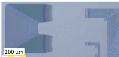
Figure 1: Microscopy image of silicon nitride arrayed waveguide grating
