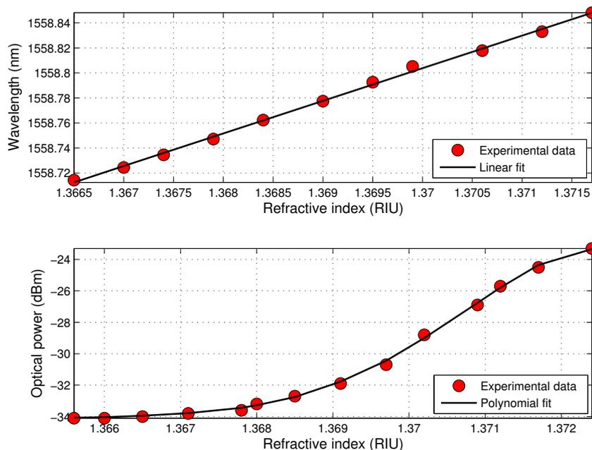
**Fig. 2:** Wavelength shift of the cladding mode around 1558.8 nm (up) and optical power change around 1559.8 nm (down).
