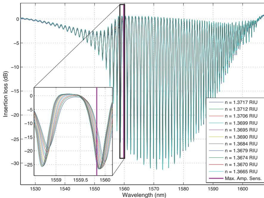
**Fig. 1:** TFBG under different surrounding refractive index conditions, with a zoom to the most sensitive mode in terms of wavelength shift (left) and insertion loss (right).
