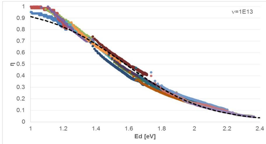
**Figure 3:** The experimental aging curves (colored) and the fitted curve (dashed) as a function of  $E_d$
