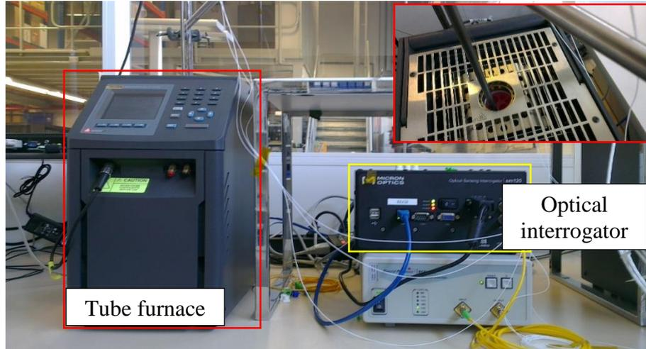
**Figure 1:** The experimental setup of the accelerated aging experiment
