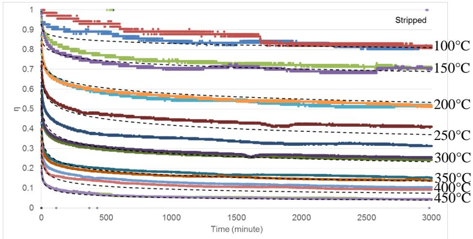
**Figure 2:** The experimental (colored lines) and the theoretical (black dashed lines) isothermal aging curves for the stripped DTGs
