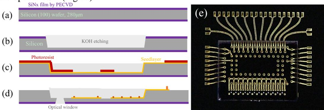
Fig. 2 process flow of silicon interposer (a) PECVD on both side; (b) KOH etching; (c) lithography on 3D structure; (d) chemically etching metal traces and 2nd KOH etching (e) finished silicon interposer.
