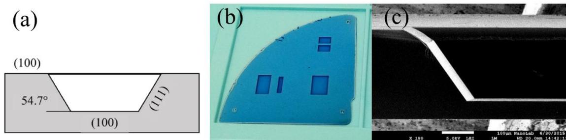
Fig. 3 (a) scheme of anisotropic wet etched profile of (100) silicon; (b) photo of 1 inch silicon wafer with etched holes, with a passive layer of  $\text{SiN}_x$ ; (c) SEM photo of cross section of etched wafer, with smoothed corner and the side wall
