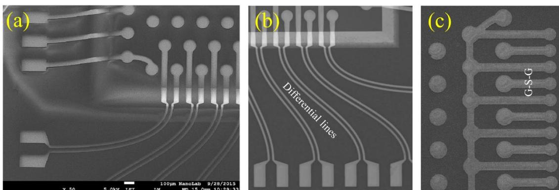
Fig. 4 (a) lithography on 3D structure; plated gold traces for defining the differential lines. Plated differential lines (b) and GSG lines (c).
