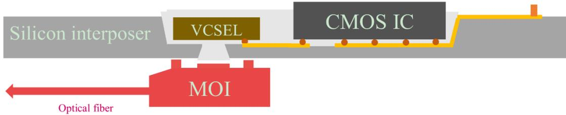
Fig.1 scheme of assembly CMOS driver, VCSEL, MOI
