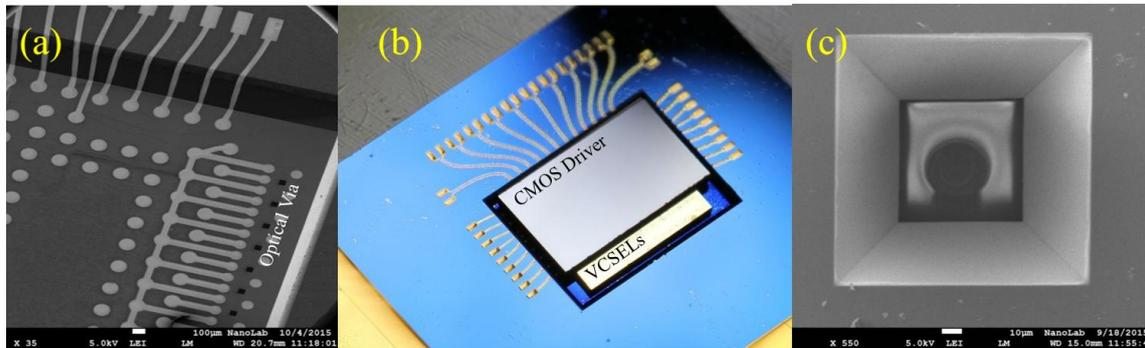
Fig. 5 (a) photography of silicon interposer (b) photo of assembled silicon interposer (c) one of 12 optical windows, opened from the backside, and active region of VCSEL.
