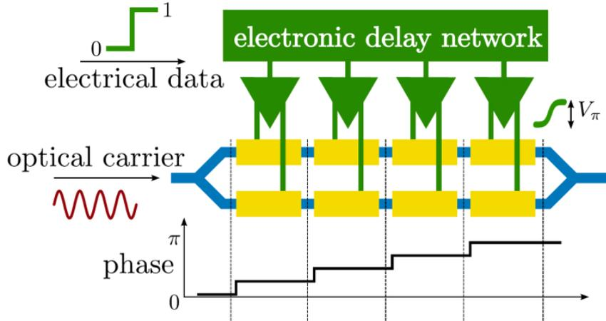
*Figure 1: Working principle of the segmented architecture*
