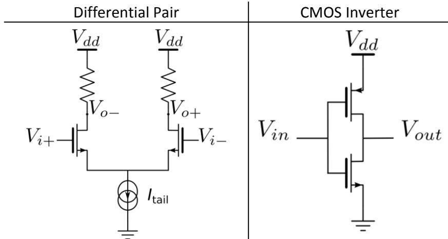
Table 1: The differential pair and the inverter as possible driver topologies
