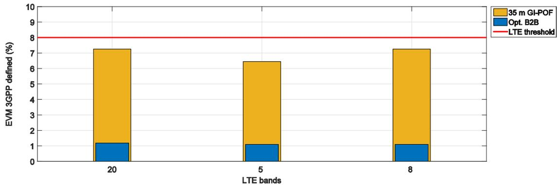
Fig. 3 LTE EVMs for different link lengths.
