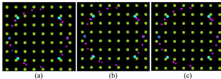
Fig. 4 Constellation diagrams for the optical B2B link of band 20 (a), 5 (b) and 8 (c). The user downlink channel with 64-QAM (green marks) and control channels (yellow, light blue, purple and red) are shown.
