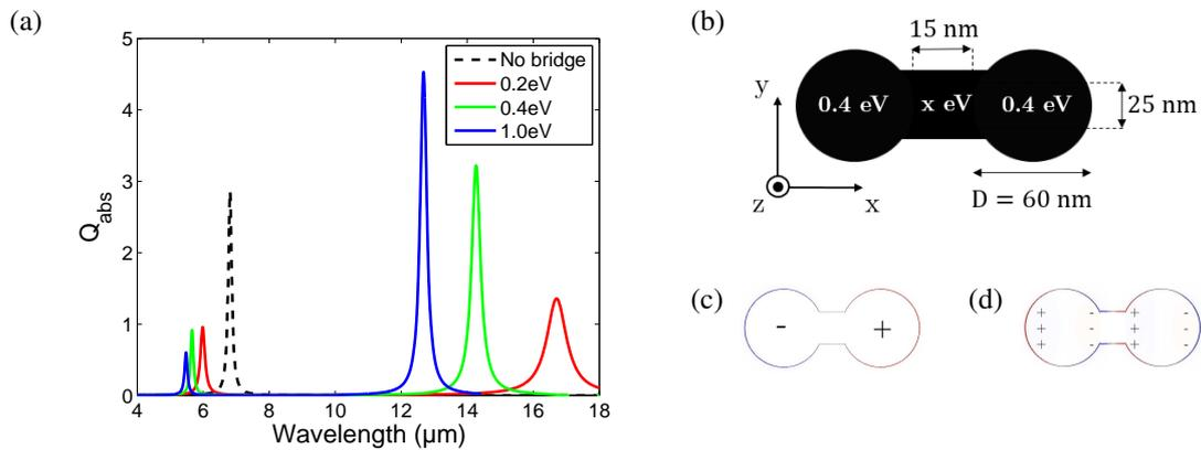
Figure 2: (a) Absorption efficiency of a graphene charge transfer dimer with varying bridge doping. The non-bridged dipolar-dipolar resonance is plotted in black dashed line for comparison. (b) Scheme of the studied structure. (c) Charge densities of the charge transfer plasmon resonance and (d) the screened bonding dipolar plasmon.
