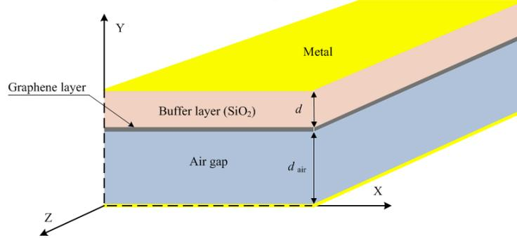
Fig. 1. Schematic diagram of PPWG with graphene and SiO<sub>2</sub> layers
