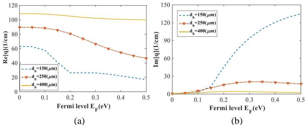
Fig. 2. Dispersion dependences of the first  $TE$  waveguide mode propagation constant versus Fermi level for  $f=0.3$  THz, for  $d_2=(150,250,400)$   $\mu\text{m}$ , for planar metal waveguide (a) the real part, (b) the imaginary part.
