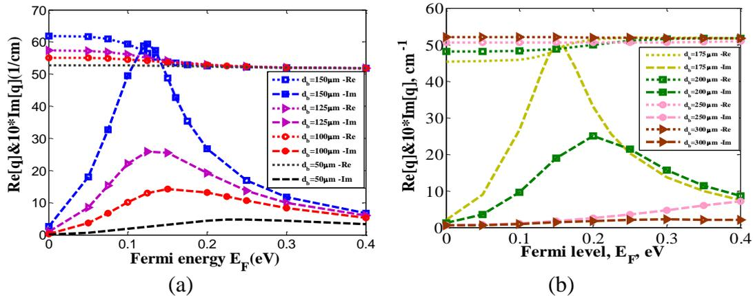
Fig.3. (a) Dependences of  $TE_{01}$  modes propagation constant versus Fermi level for different buffer thickness  $d_b$ ; real parts ( $\text{Re}[q]$ ), and imaginary part multiplied by 10 ( $\text{Im}[q]$ ), for  $f=0.3$  THz. (b) Dependences of waveguide modes propagation constants  $q$  versus Fermi level for different buffer thickness  $d_b$ ; real parts ( $\text{Re}[q]$ ), and imaginary parts multiplied by 10 ( $\text{Im}[q]$ ), for  $f=0.3$  THz.
