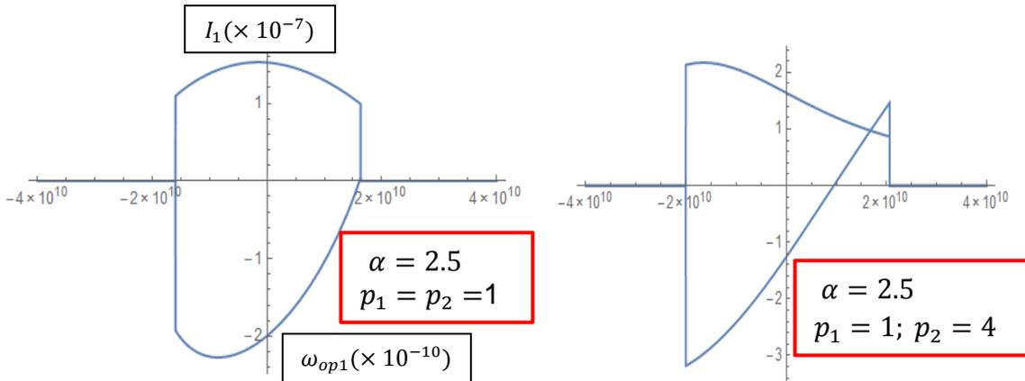
Fig.2. Calculated intensity  $I_1 (\times 10^{-7})$  and operation-frequency shift  $\omega_{op1} (\times 10^{-10})$  versus detuning  $\omega_{21} \equiv \omega_2 - \omega_1$  within the locking range for  $\alpha = 2.5$ . Left: symmetric pumping. Right: strongly asymmetric pumping.
