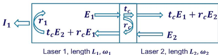
Fig.1 Schematics of coupled-cavity laser. The coupler is characterized by transmission and reflection coefficients  $t_c$  and  $r_c$ , respectively. In laser  $j$ ,  $E_j$  is the complex electric-field amplitude incident on the coupler and  $r_j$  is the reflection coefficient of the mirror opposing the coupler.
