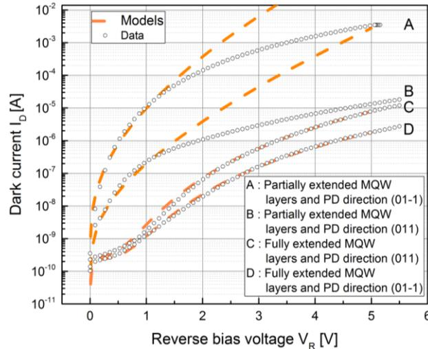
Figure 3 Open points: Measured IV characteristics for four photodetectors showing different dark current behavior. All detectors share the same design parameters, except for etch-active and direction. Orange lines: modeled dark current.
