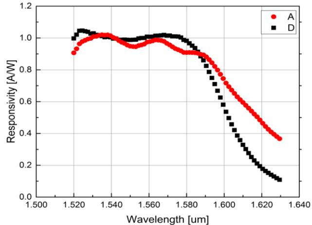
Figure 4 Responsivity of photodetectors A and D at a reverse bias of 3 V. The wavelength is swept from 1520 to 1630 nm.
