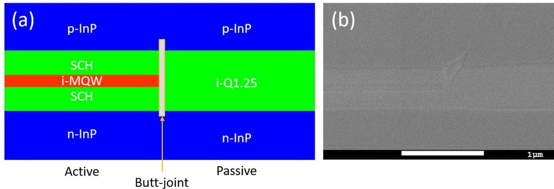
Figure 1(a) Schematic of the device. Indicated in the figure are the Separate Confinement Heterojunction (SCH) layers and the active region. At the interface of the active-passive regions, a butt-joint is formed. (b) A corresponding cross-section SEM image of a butt-joint.
