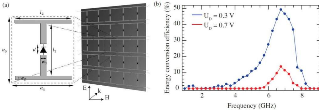
**Fig. 2** (a) Design of the metasurface energy harvester composed of cut-wire cells with an integrated diode, (b) energy conversion efficiency for different values of the threshold voltage.  $a_x = a_y = 30 \text{ mm}$ ,  $l_1 = 23.6 \text{ mm}$ ,  $l_2 = 22.8 \text{ mm}$ ,  $w_1 = 3 \text{ mm}$ ,  $w_2 = 1.6 \text{ mm}$ ,  $d = 2.95 \text{ mm}$ .
