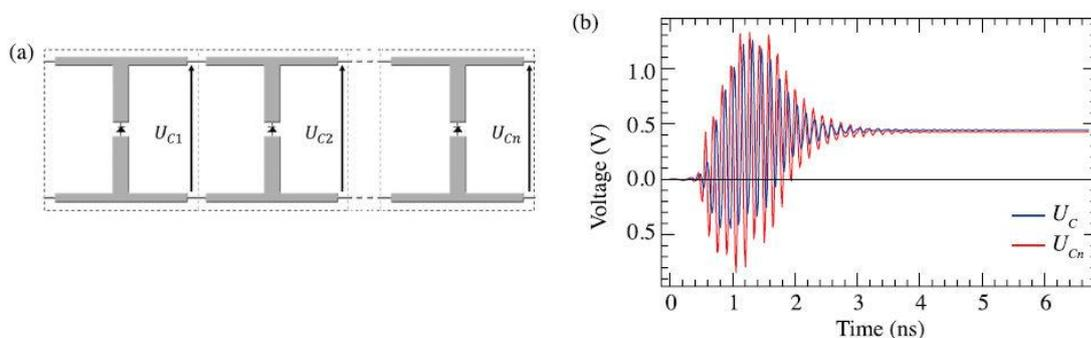
**Fig. 4** (a) Connection of the cells to channel the energy harvested. (b) Time evolution of the voltage across an unconnected cell ( $U_c$ ) and the one of a connected cell ( $U_{cn}$ ).
