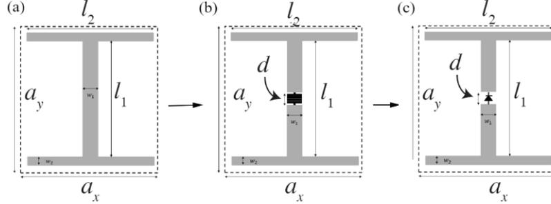
**Fig. 1** Design steps: (a) Cut-wire particle with full length, (b) cut-wire particle with embedded resistance and (c) cut-wire particle with embedded diode.
