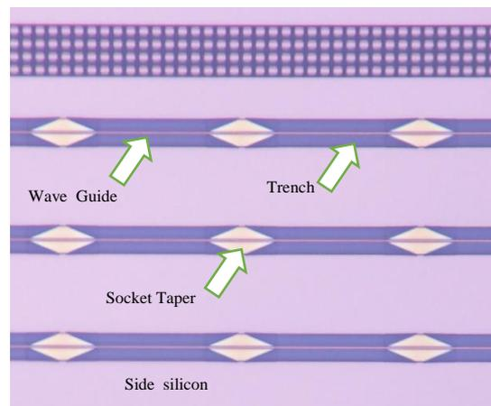
Fig. (2) Top view of SOI TE waveguide with
