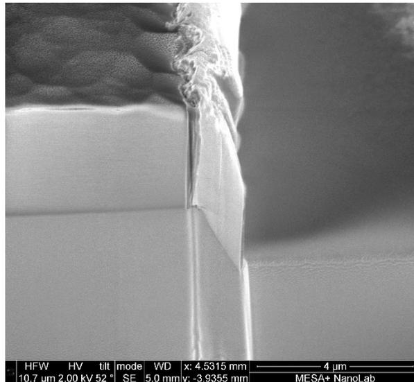
Figure 1: Severe redeposition above and on the sidewall of a KYW ridge. The thick slab on top is the residual  $\text{SiO}_2$  cladding, which was not removed before imaging.
