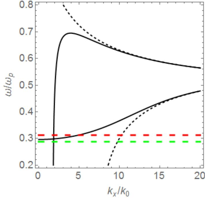
Figure 2: Dispersion of the multilayer of silver and epoxy with  $d_m = 5$  nm and  $d_d = 20$  nm. Black curves are the edges of the plasmonic band, red dashed curve is the absorption line and green curve is the emission line.
