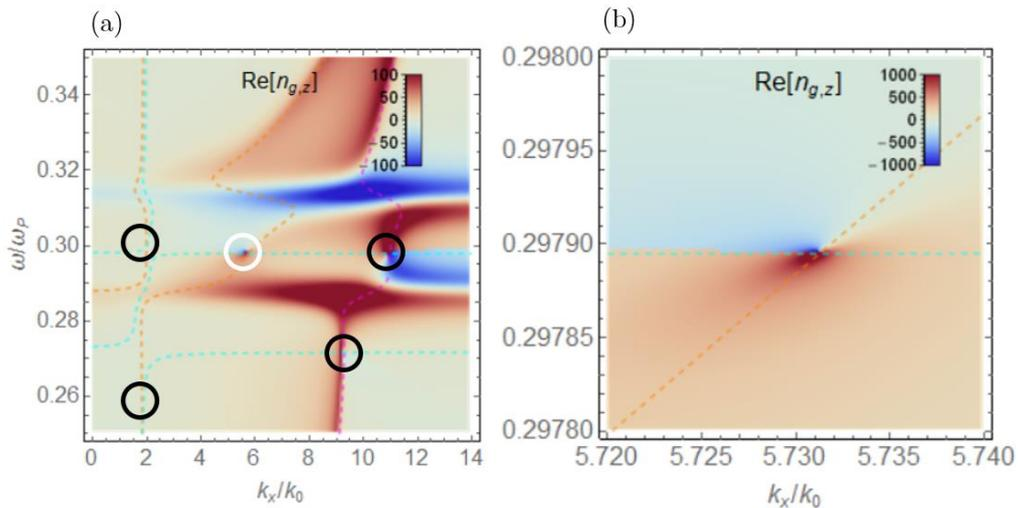
Figure 4: (a): group index in growth direction  $n_{g,z}$  of the infinite multilayer. Orange curve is the plasmonic band edge at the center of Brillouin zone, purple curve is the plasmonic band edge at the edge of Brillouin zone and cyan curve shows the region where there is loss-compensation. Circles point out the presence of exceptional points. (b) Same as (a), zoom on the exceptional point delimited by the white circle.
