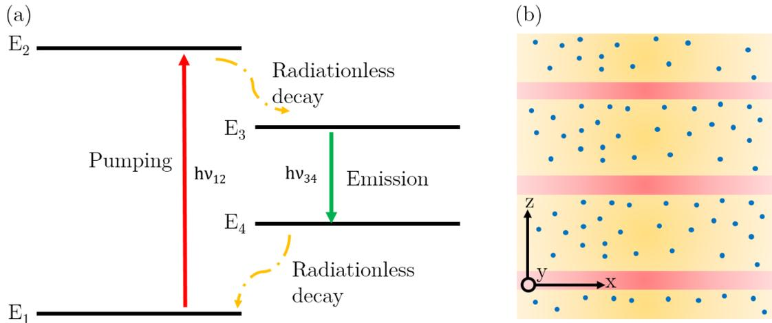
Figure 1: (a) Four-level dye scheme, with absorption line in red and emission line in green. (b) Structure under study: periodic multilayer of metal and dye-infiltrated dielectric.
