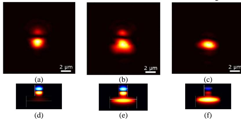
**Figure 6:** Captured images of optical field distribution at output of the antisymmetric mode converter for wavelengths (a) 1530 nm, (b) 1545 nm, and (c) 1600 nm. Simulated mode profiles (real E-field) for nominal antisymmetric mode converter design at wavelengths (d) 1492 nm, (e) 1517 nm, and (f) 1542 nm.
