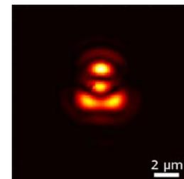
**Figure 4:** Captured optical intensity distribution of symmetric mode converter at 1570 nm wavelength.
