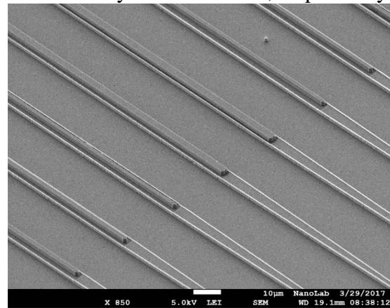
**Figure 2:** SEM image of array of mode converters of different geometries.
