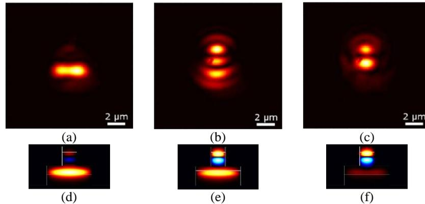
**Figure 3:** Captured images of optical field distribution at output of symmetric mode converter for wavelengths of (a) 1530 nm, (b) 1590 nm, and (c) 1600 nm. Simulated mode profiles (real E-field) for nominal symmetric mode converter design at wavelengths (d) 1492 nm, (e) 1517 nm, and (f) 1542 nm.
