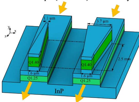
**Figure 1:** Mode converter designs (not to scale.) excitation of antisymmetric (left) and symmetric (right) super-modes. Layer thicknesses are, top to bottom, 650 nm, 1100 nm, 1000 nm, and 500 nm.
