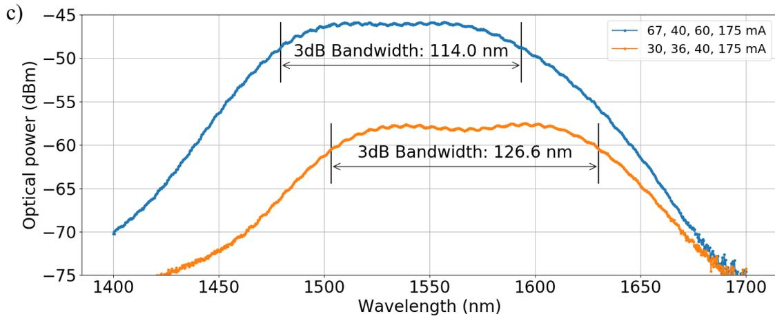
Figure 1: a) Layout of the broadband source with 4 SOAs and their respective photoluminescence peak wavelength. b) Emission spectra of each individual SOA section. c) Emission spectrum of the broadband source with maximized bandwidth for two different power levels. The legend reports the current injection used for each SOA section.
