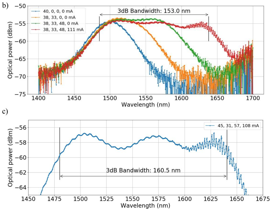
Figure 2: a) Schematic of the second broadband source design including a multimode-interference reflector (MIR) for back-reflection. b) Influence of each SOA section on the emission spectrum. c) Record bandwidth obtained with the source.
