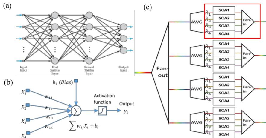
Fig. 1 (a) A 4-layer DNN structure, (b)the model of one Artificial neuron (c)schema of four neurons in one layer with SOAs and AWGs. Red rectangle: One neuron is studied in this work, with SOA 1 to 4 tuning the weight of channel 1 to 4, respectively.
