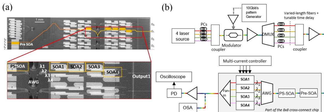
Fig. 2 (a) A micrograph of the fabricated 4:1 neuron is displayed. (b) Experimental set up to analyze the weight tuning at the neuron.
