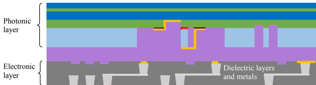
Figure 4: Schematic cross section of the bonded wafer stack
