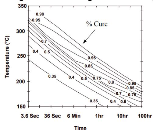
Figure 3: BCB curing function depending on time and temperature [7]
