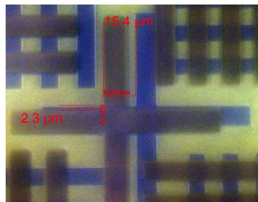
Figure 5: Alignment after bonding glass to Si, horizontal offset is due to thermal expansion
