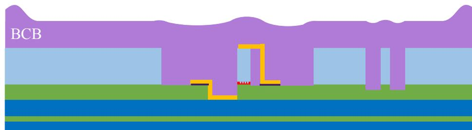
Figure 2: Schematic cross section of the InP wafer with the applied BCB including edge beads and remaining topology
