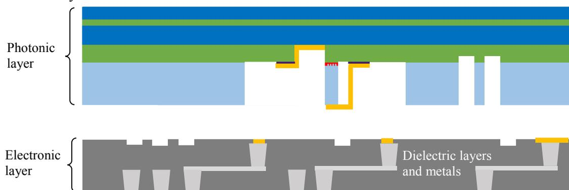
Figure 1: Schematic cross section of the photonic (top) and electronic (bottom) wafer
