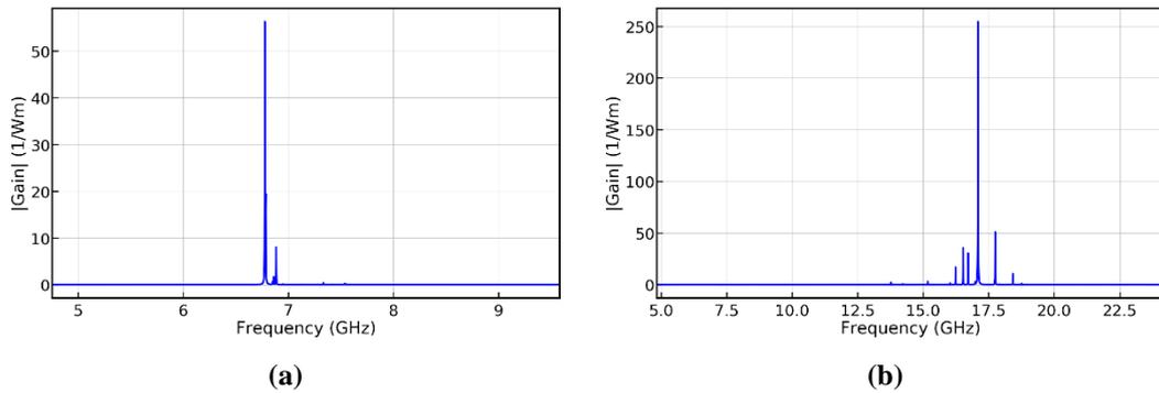
Figure 6: the calculated gain spectra for (a) the tellurite coated waveguide and (b) the suspended rib waveguide. The values correspond to  $\frac{g_0}{A_{eff}}$  as seen in Eq. (1).
