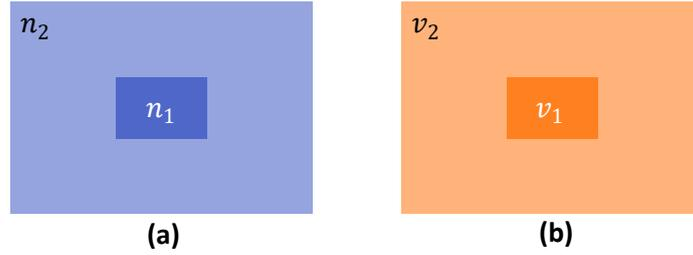
Figure 2: Schematic drawings of (a) an optical waveguide ( $n_1 > n_2$ ) and (b) an acoustic waveguide ( $v_1 < v_2$ ). Here,  $n_i$  is the refractive index of the material, and  $v_i$  is the speed of sound of the material.
