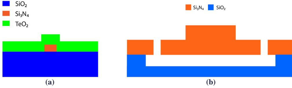
Figure 3: Schematic drawing of (a) the TeO<sub>2</sub> coated Si<sub>3</sub>N<sub>4</sub> waveguide, (b) suspended silicon nitride rib waveguide.
