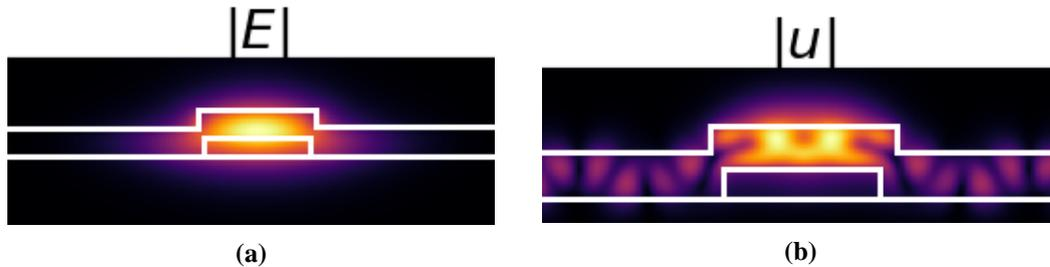
Figure 4: Simulated modes of the TeO<sub>2</sub>-coated Si<sub>3</sub>N<sub>4</sub> waveguide, with (a) the electric field showing the optical mode and (b) the displacement field showing the acoustic mode.
