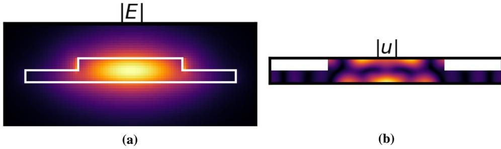
Figure 5: the simulated modes for the suspended rib waveguide, with (a) the electric field showing the optical mode and (b) the displacement field showing the acoustic mode. of sound between the materials, as the interaction requires the wavelength of the optical and acoustic wave to be similar.
