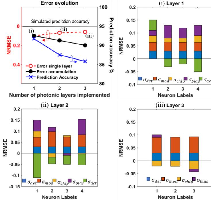
Fig. 2 Top left: the error evolution and prediction accuracy vs. number of photonic layers implemented. The error contribution analysis in (i) Layer 1, (ii) Layer 2, and (iii) Layer 3, resulting in an average error of single layer shown on top left.
