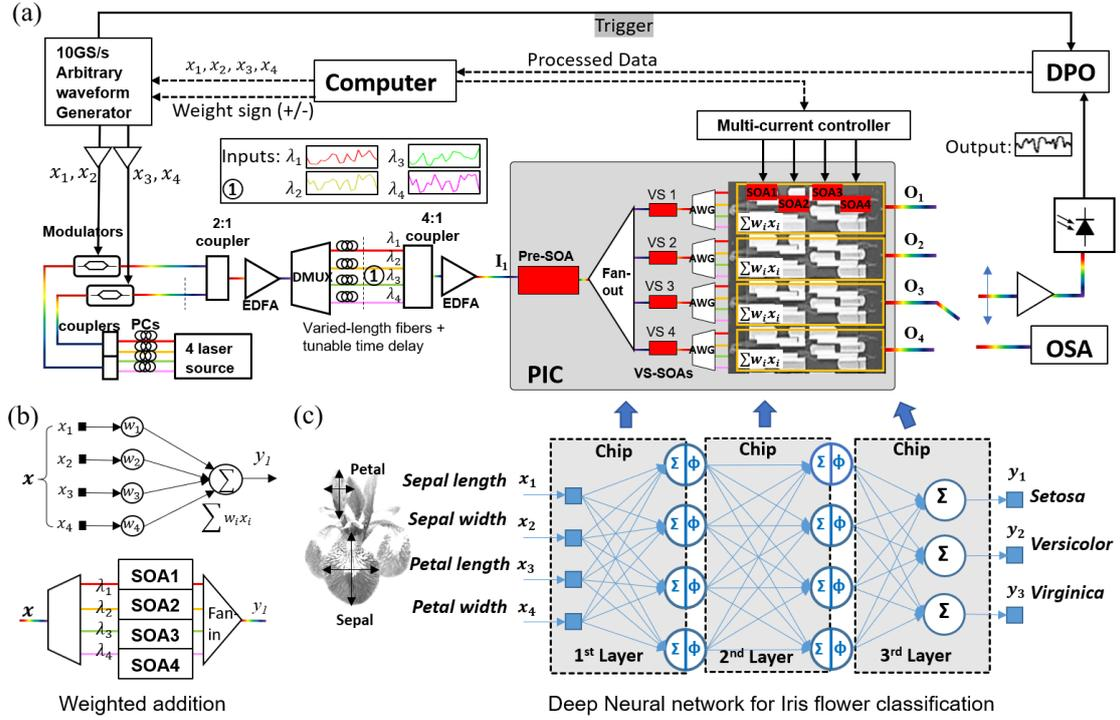
Fig. 1 (a) The experimental setup. (b) Weighted addition in the artificial neuron model and the corresponding photonic implementation. (c) Three-layer deep neural network for image classification, with reconfigurable photonic layer in gray box.
