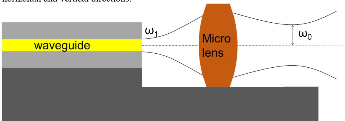
Figure 1. The model of the waveguide coupling system with micro-thin lens
