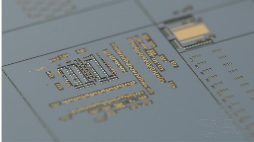
Figure 2: Picture of the InP based photonic membrane layer with windows to access and interconnect the photonic (gold) and the electronic contact pads (aluminum). Photo by Florian Lemaitre
