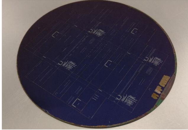
Fig. 1: Photonic wafer (BiCMOS wafer with InP membrane) with SiO<sub>2</sub> hard mask (dark blue) for etching windows into the InP membrane
