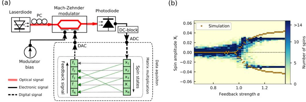
Figure 1: (a) Experimental setup of an OEO-based CIM. (b) Distribution of spin amplitudes for  $N=100$  uncoupled OEOs as the feedback strength is increased. Orange dots indicate the maximum of the distribution obtained from simulating eq. (2). Adapted from [1].
