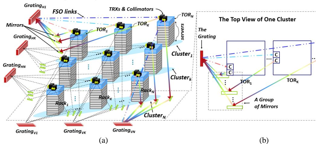
Fig.1: (a) The optical wireless DCN architecture based on passive diffractive optics and fast tunable lasers; (b) The top view of one cluster of the optical wireless DCN; C: Collimator
