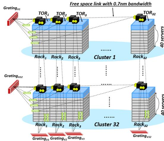
Fig.2: The optical wireless DCN architecture with 32\*32 racks interconnected
