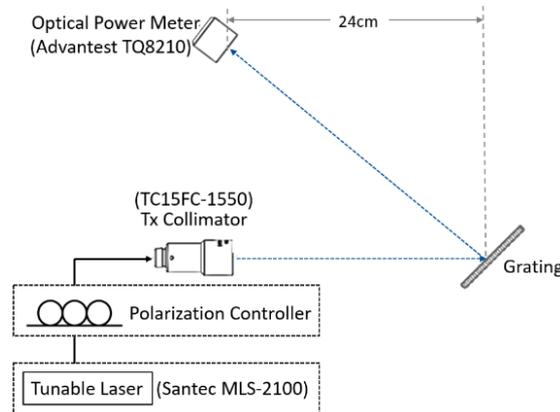
Fig.2: Experimental setup for power loss measurement
