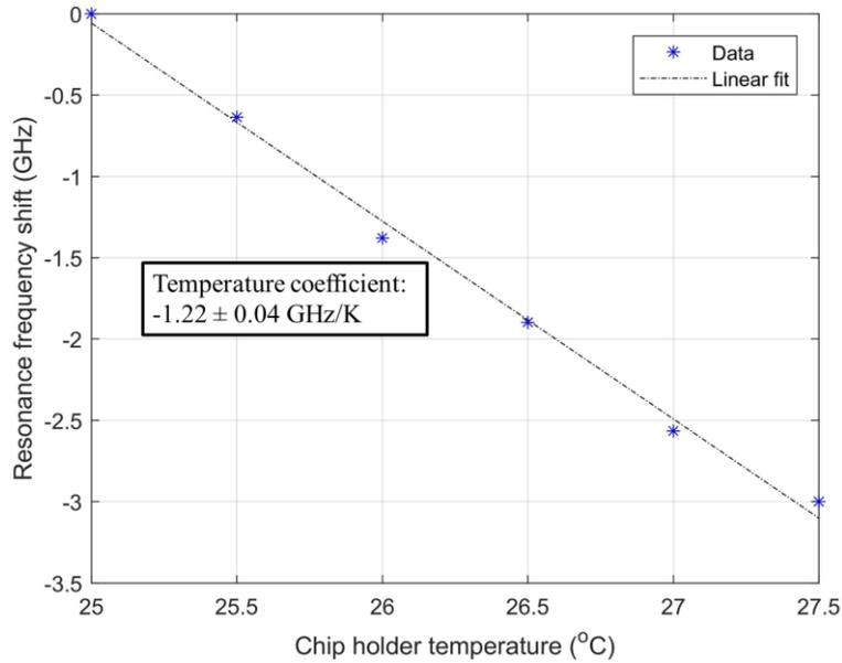
Fig. 3. Laser cavity temperature coefficient calibration.
