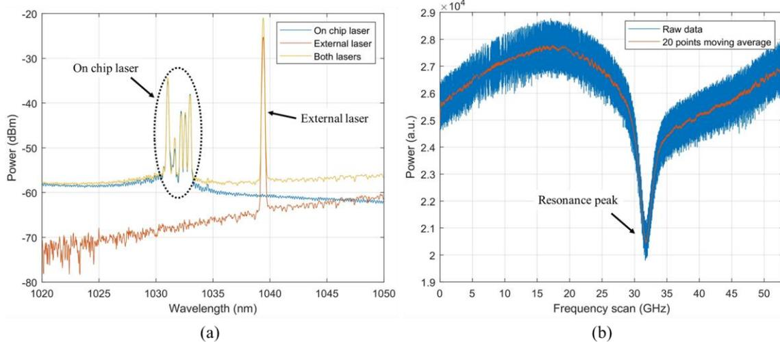
Fig. 2. (a) Optical spectra of the on-chip laser alone, Toptica laser alone pass through the chip, and both of them at the same time. (b) Piezo scan of the Toptica laser across one of the ring cavity resonances. The center wavelength is set to 1040.970 nm, and the full piezo scan range is 53 GHz ( $\sim 0.19$  nm).
