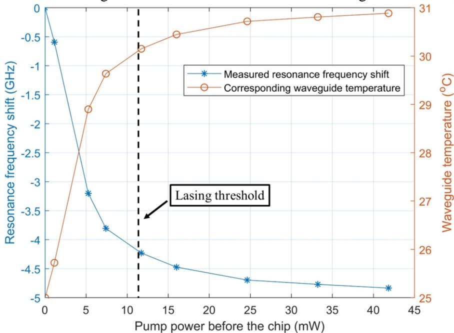
Fig. 4. Resonance frequency shift and the corresponding waveguide temperature as a function of pump power before the chip. The lasing threshold is 11.3 mW and marked with a dashed vertical line.
