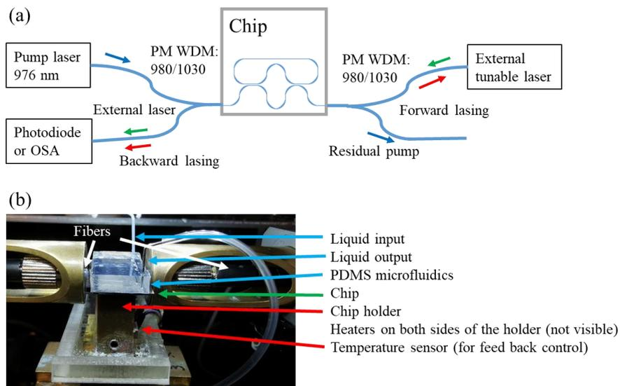
Fig.1 The experiment setup. (a) The setup layout. Pump (976 nm) light is indicated with blue arrows. On-chip lasing is indicated with red arrows. The external tunable laser light is indicated with green arrows. (b) Image of the setup around the optical chip during experiment. The fiber coupling to the chip, the microfluidics on the chip, and the temperature control components are indicated in the image.
