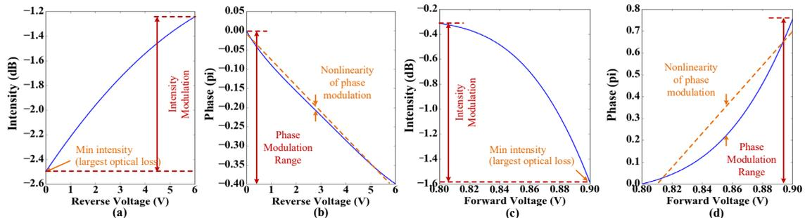
Fig. 1 (a) Measured intensity modulation and (b) phase modulation response of the used depletion modulator model (0 V to 6 V); (c) Measured intensity modulation and (d) phase modulation response of the used injection modulator model (0.8 V to 0.9 V).
