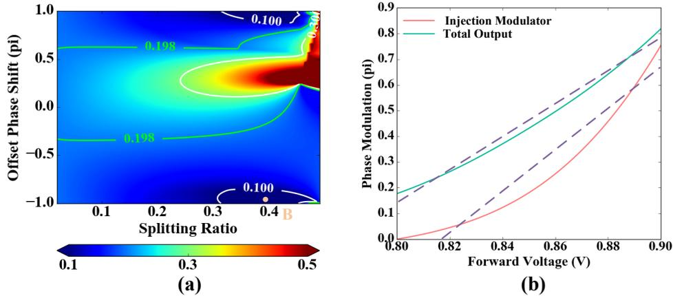
Fig. 4. PIN based injection modulator simulation. (a) Simulation results for sweeping coupling ratio and phase shifts; (c) Phase response of the configurable modulator at  $\kappa = 0.4$  and  $\phi_s = -0.9\pi$ .
