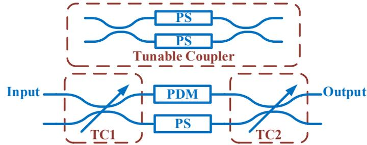
Fig. 2 Structure of the configurable modulator. PDM: plasma dispersion modulator; PS: phase shifter; TC: tunable coupler.
