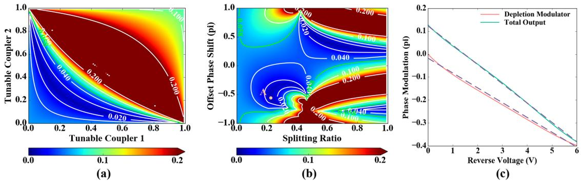
Fig 3. PN based depletion modulator simulation. (a) Simulation results for sweeping coupling ratio of both tunable couplers from 0 to 1 with a fixed phase shift  $\phi_s = 0$ ; (b) Simulation results for sweeping coupling ratio and phase shifts; (c) Phase response of the configurable modulator at  $\kappa = 0.24$  and  $\phi_s = -0.57\pi$ .
