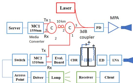
Figure 1: Simplified block diagram of the end-to-end RoF LiFi network. MC: Media Converter, PD: Photodiode, MPA: Medium Power Amplifier. LNA: Low Noise Amplifier. CDR: Clock- and Data-Recovery.
