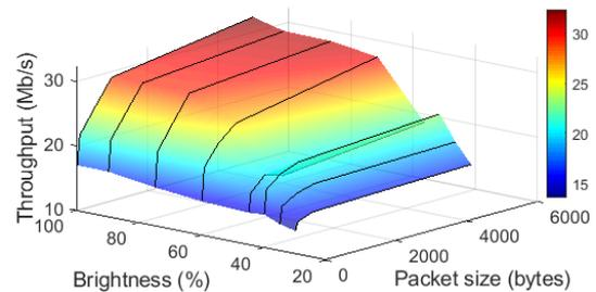
Figure 2: Transmission data rate in function of both brightness and packet size.
