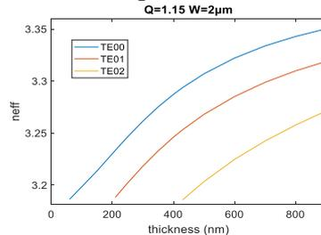
Figure 2 Effective index for different TE-modes as function of thickness for  $Q=1.15\mu\text{m}$  and  $W=2\mu\text{m}$
