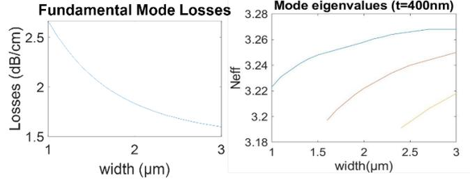
Figure 3 Optical loss for the fundamental mode  $TE_{00}$  and effective indices of the first three eigenmodes as function of width of a shallow etched ridge waveguide with thickness=400 nm
