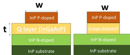
Figure 1 Schematic for the ridge waveguide in both shallow and deep etched technology
