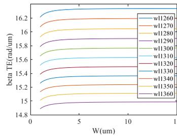
Figure 5 Propagation constants for the deep etched straight waveguide.
