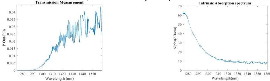
Figure 4 a) Measurement of transmission spectrum of a straight waveguide (4 mm long) with uncoated end facets close to the quaternary alloy bandgap, Q=1.25 $\mu\text{m}$ . b) Measured absorption coefficients as a function of wavelength.
