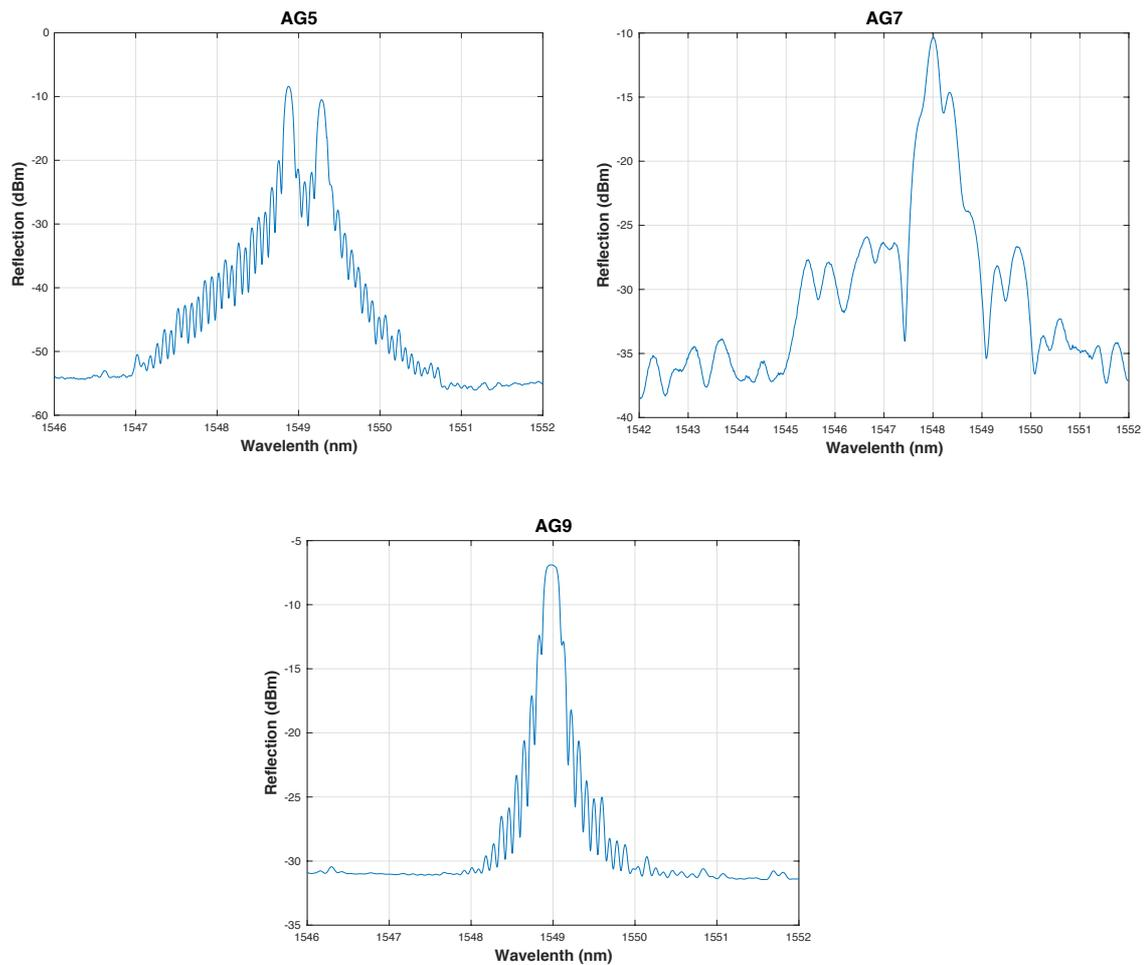
Figure 3. Reflection spectra of the gratings before the exposure.
