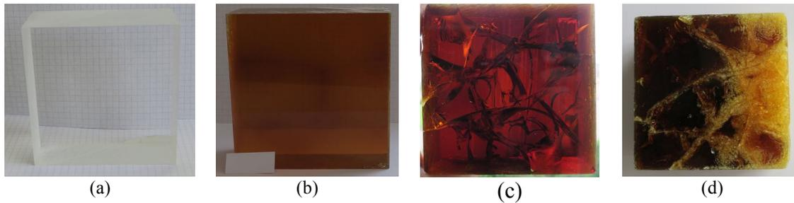
Figure 2 PMMA block (a) before irradiation, (b) after 250 kGy, (c) 1 MGy, (d) 2 MGy.
