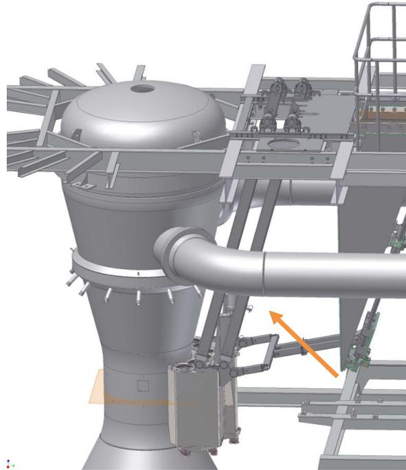
Figure 1 Poseidon facility at BR2. The rotation motor compartment is indicated by the arrow. It is located in the pool ~1.8 m above the reactor mid-plane.
