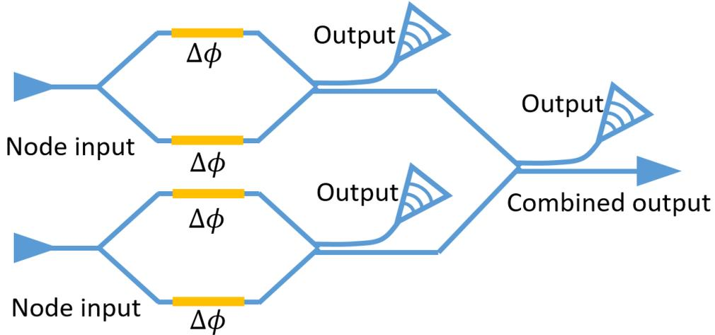
Figure. 1. Illustration of proposed easy observation readout architecture, consisting of 2 channels and one combiner.
