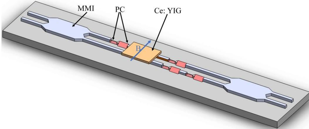
Fig. 1 Schematic of the circulator
