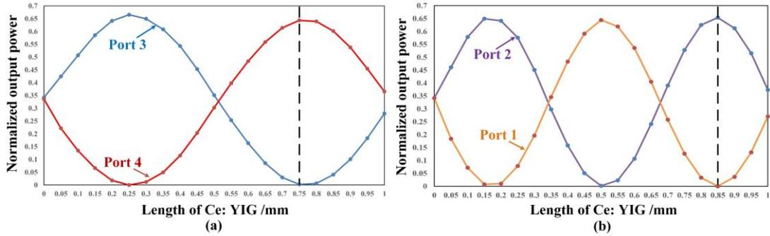
Fig. 3 Normalized output power distribution as a function of the length of Ce: YIG, for a TE polarized input signal. (a) In forward direction with input at port 1 (b) In backward direction with input at port 4
