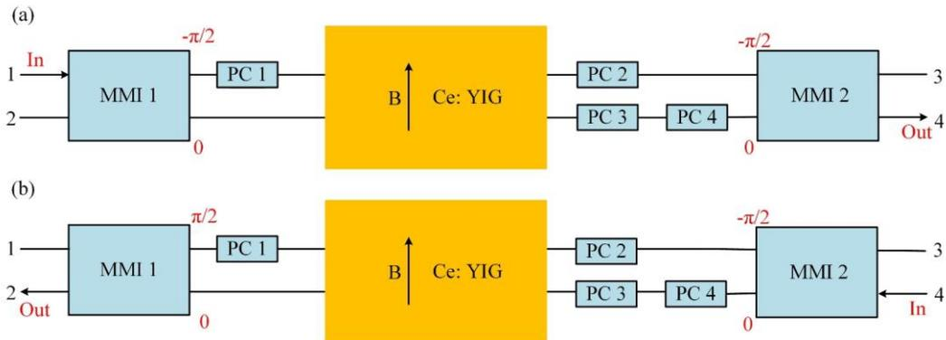
Fig. 2 Schematic diagram of the circulator (a) Forward direction (b) Backward direction
