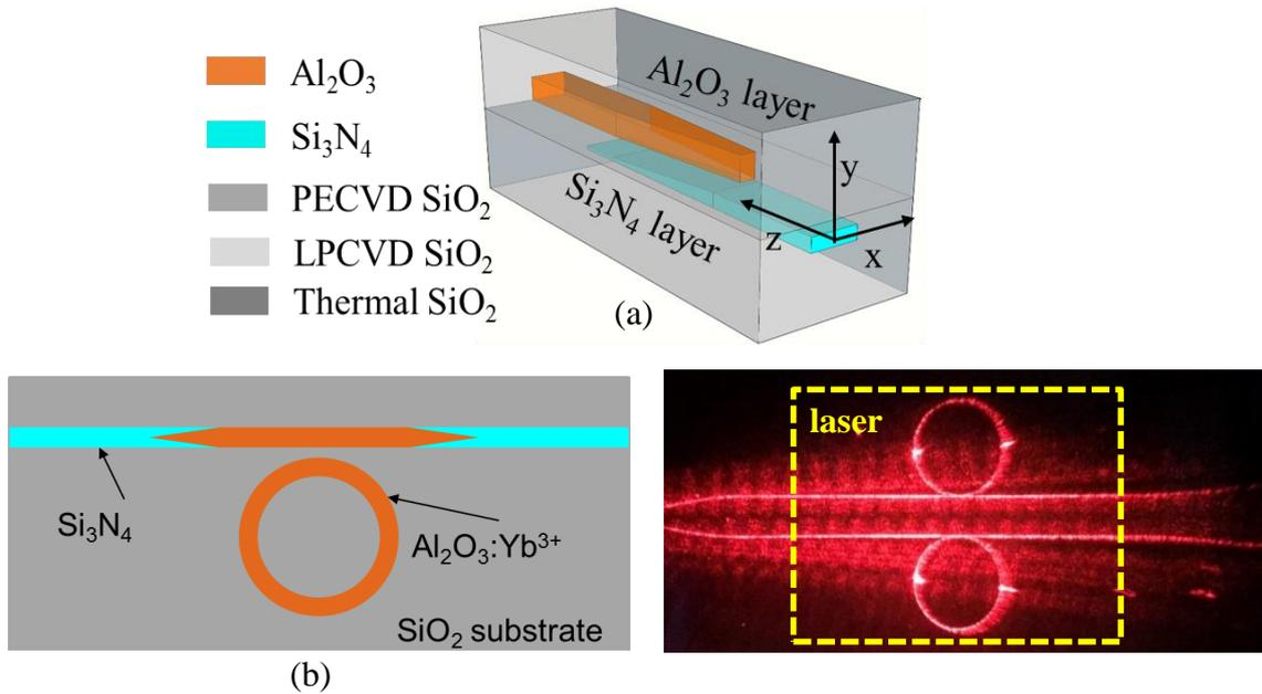
Fig. 1. (a) 3D schematic of the vertical coupling region [17] and 2D schematic of the integrated Al<sub>2</sub>O<sub>3</sub>:Yb<sup>3+</sup> microring laser in the Si<sub>3</sub>N<sub>4</sub> platform with tapered waveguides in the vertical coupling region. (b) Mask layout of the integrated lasers, with integrated 3 dB 975.5 nm pump power splitter, and its optical image aligned using the red light laser.
