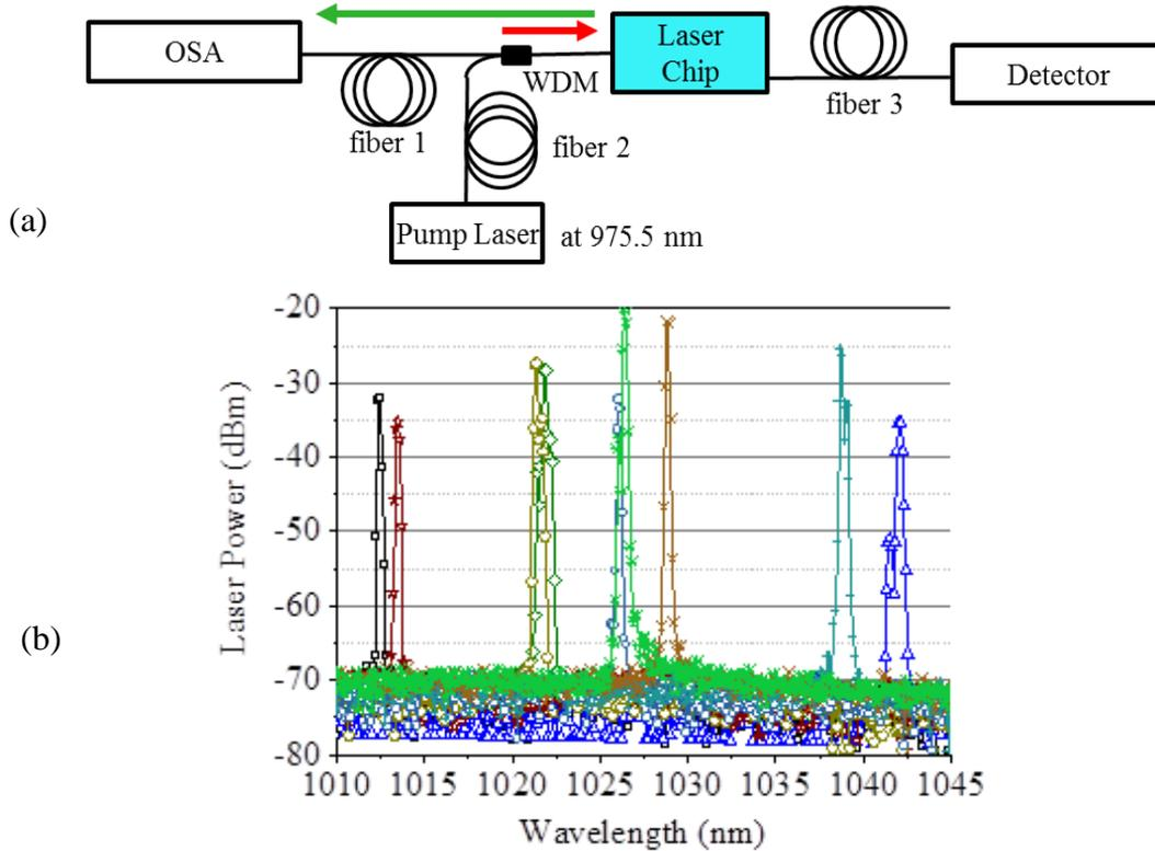
Fig. 2. (a) Schematic of the experiment setup based on fibers. The lasers are optically pumped using an external diode at 975.5 nm wavelength. (b) Measured lasing peaks near the peak emission of  $\text{Yb}^{3+}$  at the wavelength of 1030 nm, including a schematic of the integrated  $\text{Al}_2\text{O}_3:\text{Yb}^{3+}\text{-Si}_3\text{N}_4$  microring (MRR) laser. Different colors indicate that the measurements are from different integrated MRR lasers.
