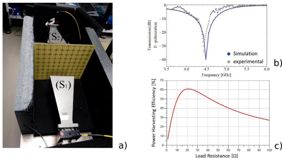
**Fig. 1** (a) Cut-wire metasurface 10×9 in free space, (b) Transmission profile of the metasurface with E-polarization configuration (simulation and experiment), (c) Power harvesting efficiency: RF to DC conversion.
